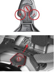
Set the contact pressure with a 1- or 2-cent coin with the adjustment screw. Stronger (+) or less (-).
